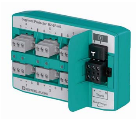
Fig. 3: R2 Segment Protector – The short-circuit and energy limiting fieldbus coupler. A separator wall creates the 50 mm thight-string-length between trunk and spurs, the intrinsically safe Ex ic circuits.
